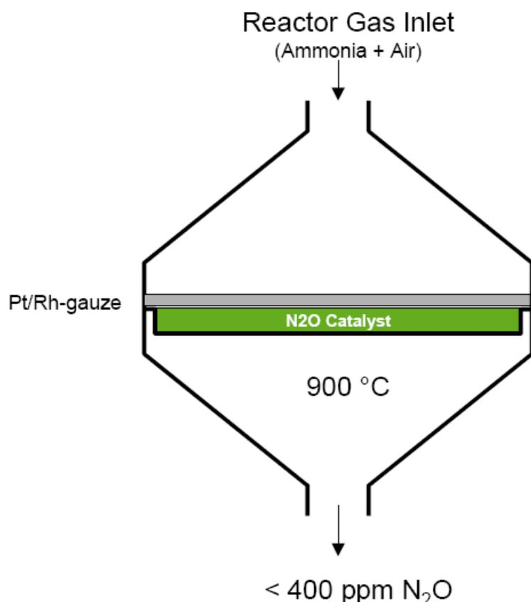
Figure 3. The diagram above depicts a typical installation of a DeN<sub>2</sub>O Secondary Catalyst.
