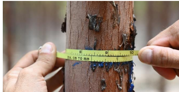
Fig 2: DBH measurement using diameter tape
